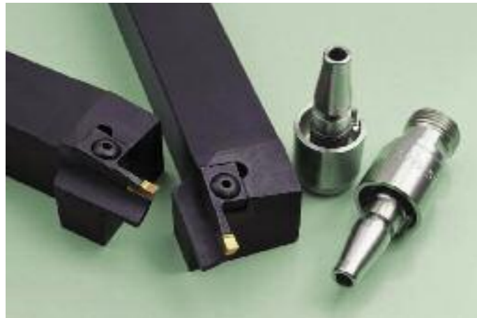
ACT2.2 tooling for face-grooving stainless steel components for medical equipment
