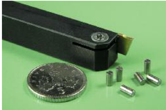
Microcut tooling for parting-off radio-metal components
