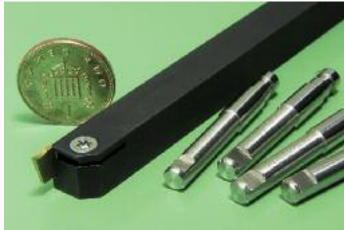
Microcut RHSS-1010 tooling used for parting-off 5mm diameter stainless steel bar
